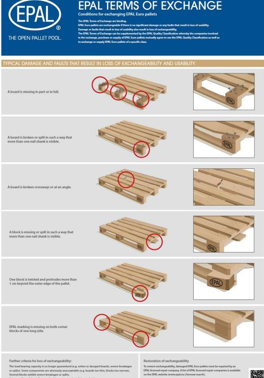
The load bearing capacity is no longer guaranteed (e.g. rotten or decayed boards, severe breakages or splits). Some components are obviously unacceptable (e.g. boards too thin, blocks too narrow). Several blocks exhibit severe breakages or splits. Several blocks exhibit severe breakages or splits. Severe soiling of the pallet may lead to contamination of the payload.
